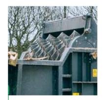
Intelligent feed wheel with lift and downward assist Variable speed linked to engine load and/or engine RPM
