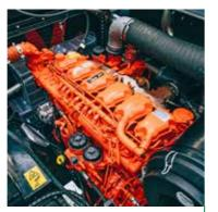
368kW (493HP) Scania DC 13 Stage V Unrivalled service access Direct drive rotor for efficient shredding
