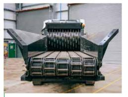
Heavy duty open-ended drag chain feeder
