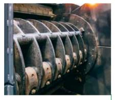
1000 RPM upturn rotor 30 swinging hammers 1,490mm (length) x 1,100mm (diameter) Single piece solid or replaceable tip hammer options
