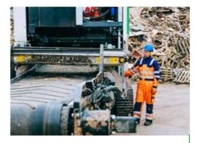
Product conveyor discharge height - 4.6m Modular design reducing downtime Lowers to ground level for maintenance access
