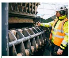
Safety interlocked access door for operator safety Electric/Hydraulic Raise/Lower of screen for ease of access Excellent rotor and anvil access for inspection and maintenance
