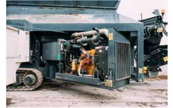
Swing out engine cradle providing operators with unrivalled maintenance access
