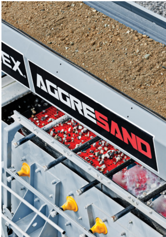
Aggregate Screen Fitted with Isolated Spraybars
