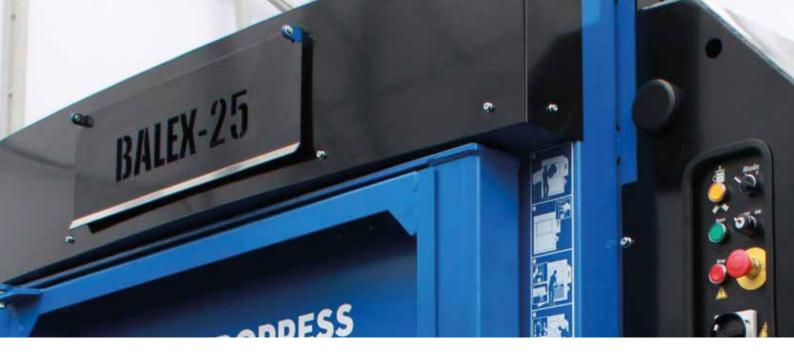
Europress Balex-25 is a compact vertical baler for wide range of uses. With its 25 tons compressions force, Balex-25 produces very dense bales weighing up to 300 kg. The cross cylinder design of the baler ensures a small footprint. With its low overall height of just 1,950 mm, it is easy to place in limited space.
