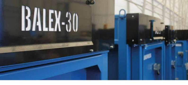
Europress Balex-30 is a compact vertical baler designed for heavy use. It is suitable for wide range of uses. The dual-mode function optimizes compression set up for different materials. With its 30 tons compression force, it produces very dense bales weighing up to 320 kg. Due to its compact cross cylinder design, the baler is easy to place in any working environment.
